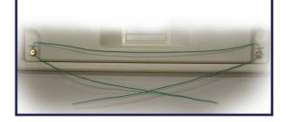
Pass the two ends of the wire through the holes of the seal, so that on the other side may emerge at least 3/4 cms both ends.
