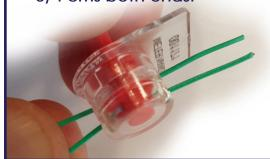
Rotate the drum flag clockwise until the inside of the rotor is completely filled with wire and the rotor no longer can be rotated.
